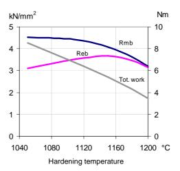
Tempering 3 x 1 hour at 560°C Dimension of test piece ∅ 4.7 mm
